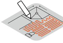
Plan the installation and chalk where each run should go to ensure you have the correct size system. Now start to lay the mat taking care not to cut or damage the mat with sharp tools. Wear soft-soled shoes throughout.
