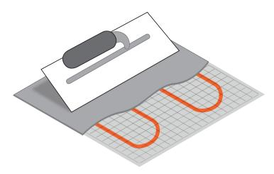
Now the mat is rigidly fixed to the sub-floor we highly recommend that you cover the cable with a thin suitable flexible levelling compound or flexible tile adhesive. We suggest testing the system again at this stage. Check with your supplier for the levelling compound and/or tile adhesive suitability for use with underfloor heating and the sub-floor.
